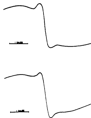
Figure 2. Collapsed esr spectrum of the N\cdot^- (glyme) \text{Na}^+ loose pair showing the presence of two species: one exchanging faster, the other slower. Lower curve: computer simulation of the spectrum.
